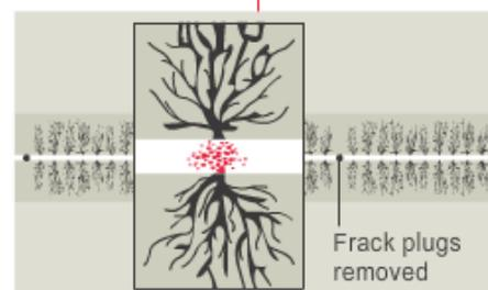
A temporary plug is inserted. The process of perforating and fracking may be repeated. Finally, the plugs are drilled out and the gas flows to the surface
