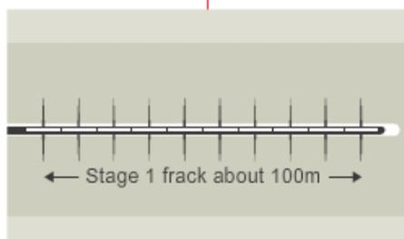
The well bore is lined with concrete to prevent fluids seeping out. Holes are perforated in the casing and shale by firing down an electric current
