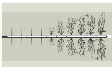
A water and sand mixture is pumped under high pressure down the well bore and into the holes where it fractures the shale. Gas in the rock is forced into the well bore
