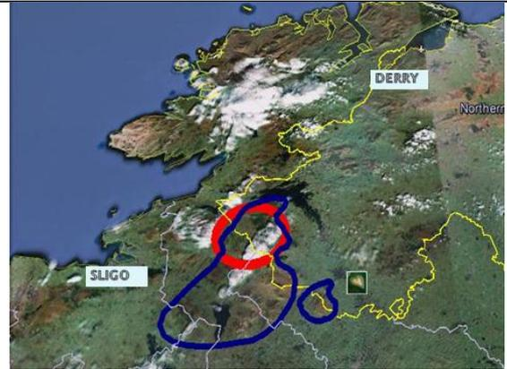
This image gives an indication of the density of pads throughout the target area of Leitrim and Fermanagh if 120 pads are constructed there. It does not show access roads, gas pipe networks or other installations.
